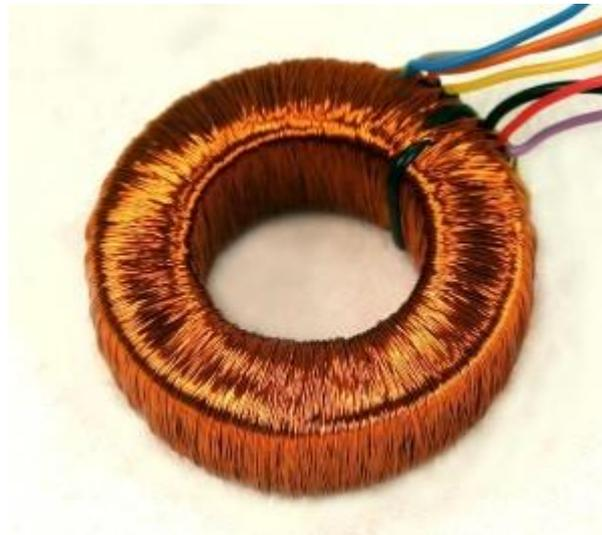
2) Something like this, only winding was made one turn clockwise around the main axis of the torus and then against to compensate for the magnetic field of one turn with current around the main axis of the torus and fully compensate the potential of the electric field between the beginning and the end of the winding. Winding around the minor axis of the torus was performed in the same direction in both cases, so that the magnetic flux "F"
